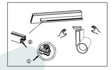
4 After finishing assembly,rotate to the desired position and turn on
